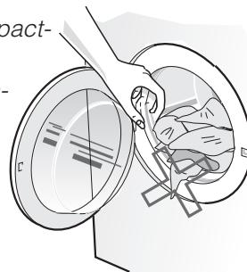
Close the door using a light pressure. Check that none of the items have become trapped between the door and the gasket.
